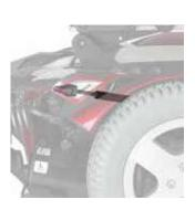
**Stability Lock Stability Lock** comes into play when base and front castors start tipping forward in relation to the rear castors, providing stability and safety.
