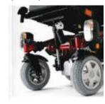
Standard Seat Tilt Seat angle can be set by a spindle or adjusted electronically for greater stability and improved downhill comfort.
