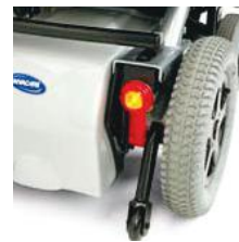
Rear wheels 14" pneumatic rear wheels with studded profile.
