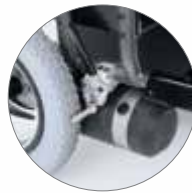
Four poles motor
